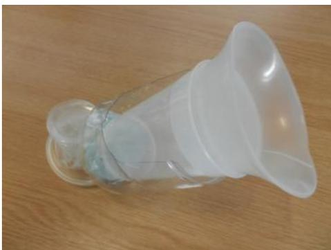
An initial prototype was made using two cut up plastic bottles and a whole packet of Bluetack. Although this design showed promise, the 'Bluetack dock' lacked sufficient rigidity to stand up to everyday use. Also, due to its 'blue peter' style appearance it was accidentally thrown away by the cleaner!
